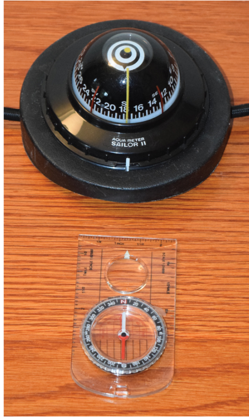
Photo 1.16 Deck compass and handheld orienteering compass WAYNE HORODOWICH
