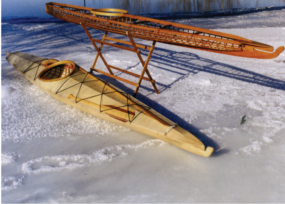
Photo 14.11 Modern custom-built replica of original one-hole baidarka taken from Atka on the Aleutian Islands. For those romantics who hanker after the “old” days, there are now a growing number of craftsmen who will build for you an original design in the traditional manner. In this beautiful model by R. Bruce Lemon of Idaho, the frames are lashed together with waxed polyester instead of sinew. The skin is made from dead 14- or 26-ounce nylon instead of the skin of a dead seal. This cover is then sewn together with braided nylon. R.
