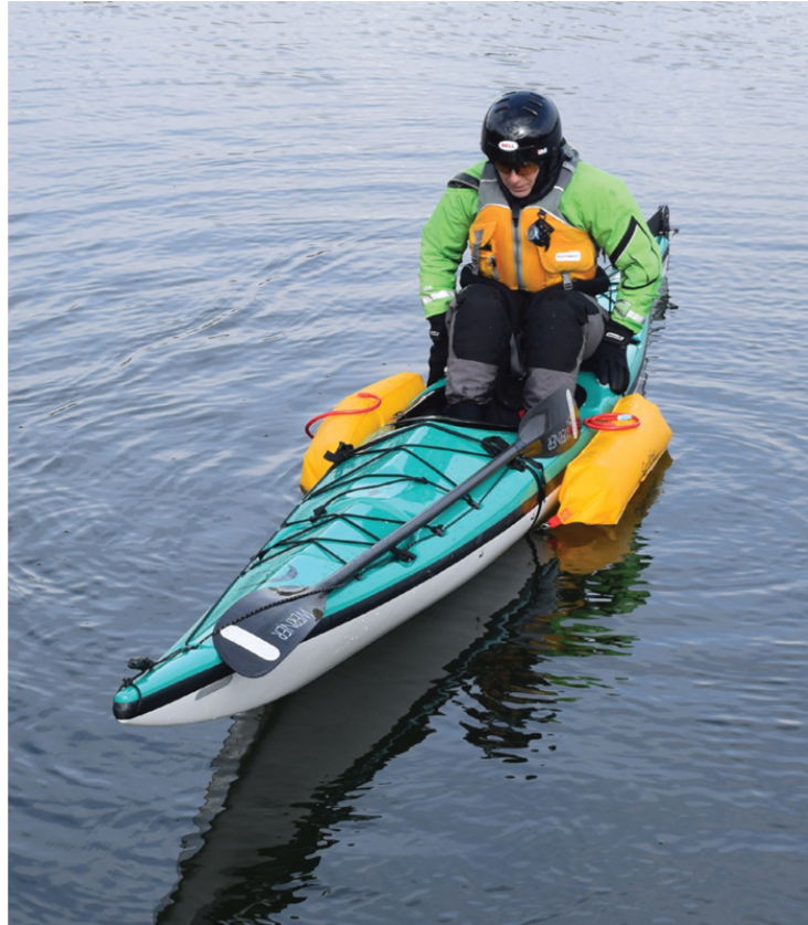
Photo 2.19 Sea Wings provide stability in both directions. Here the paddler sits on her back deck just to demonstrate the added stability. WAYNE HORODOWICH
