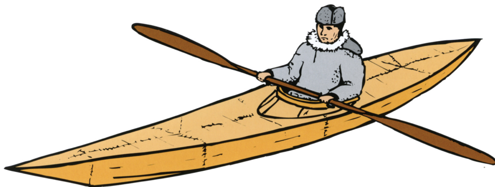
Figure 14.1 North Greenland/Hudson Bay kayak. This kayak is rather ugly when compared with other Greenland kayaks. The wide deck is flat except for the sheer up to the large round cockpit. Note the high wooden coaming. The man appears to sit quite loosely and slumped back. The paddle, drawn to scale, is long by Eskimo standards. In the photo that inspired this drawing, what appears to be a large full dustbin is stood on the deck just forward of the cockpit; this may give some indication of the stability of this particular kayak.
