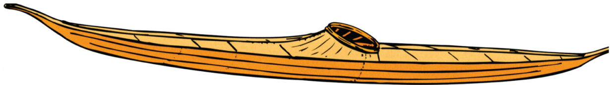
Figure 14.6 Caribou kayak (west Hudson Bay). Length: 18 feet 6 inches; width: 21 inches; cockpit: 18 inches diameter
